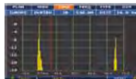
Impulse response (ECHO in COFDM TV)
